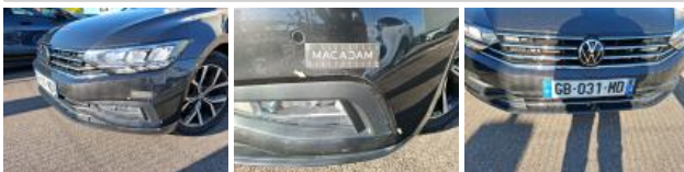
Bumper F, Crack, Repair and paint (complete)
