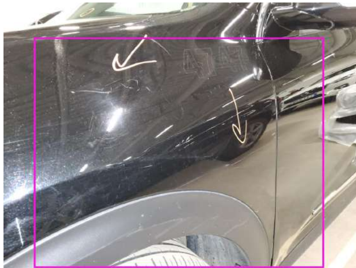
19. Fender / Front Left Paint / Scratch / Scuff
