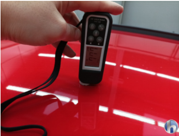
1. Roof Subsequently painted - Without repair
