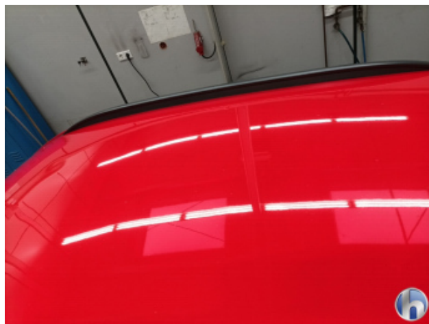
1. Roof Subsequently painted - Without repair
