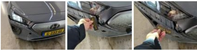
Shutter / cover F, Missing, Replace
