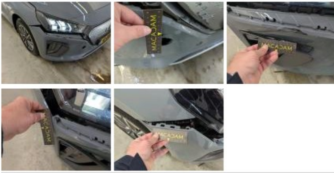
Bumper grille FR, Broken, Replace
