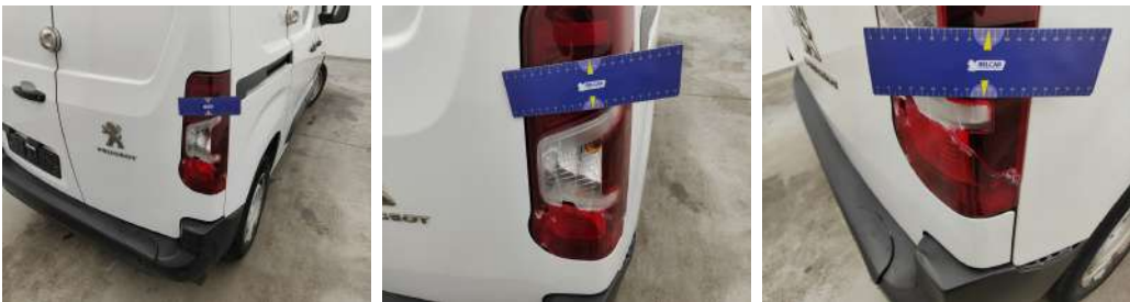
Light / Rear Right / Replace-cracked
