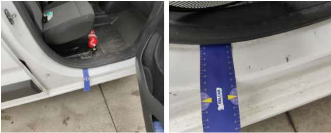
Rocker Panel Right // Smart Repair Medium-scratch + dent
