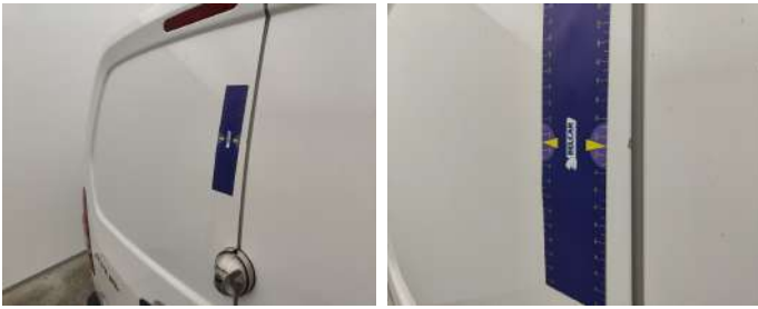
Rear Loading Door Left // Repair & Painting-scratch + dent
