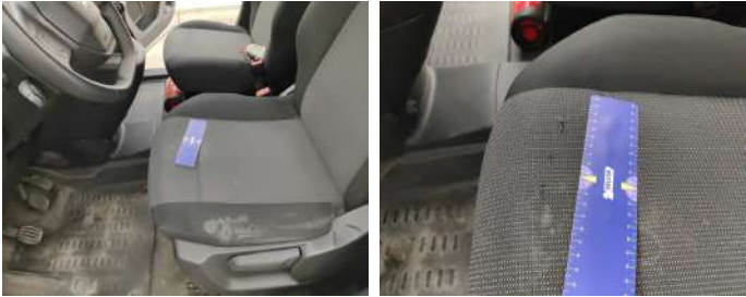
Seat Front Left / Bottom Coating / Replace-worn
