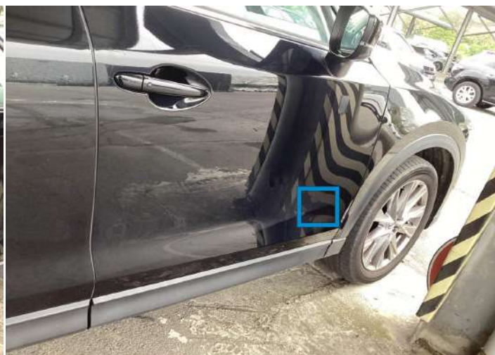
18. Door / Front Right Paint / Chipping -
