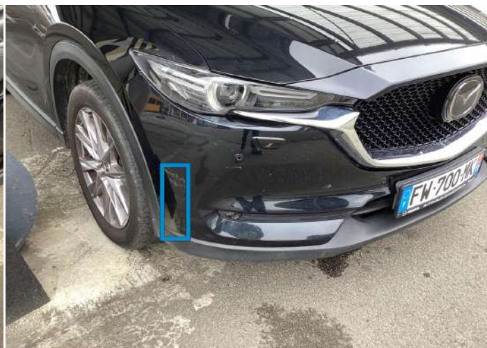
16. Corner Bumper / Front Right Paint / Chipping -
