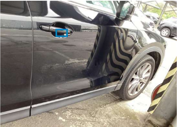
19. Door / Front Right Paint / Chipping -
