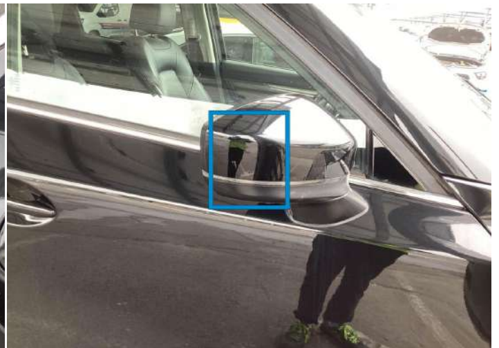
10. Mirror / Front Right Paint / Chipping -
