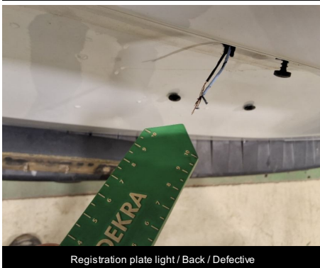
Registration plate light / Back / Defective
