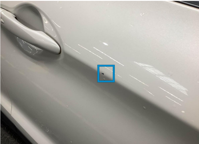
3. Door / Front Right Paint / Chipping -
