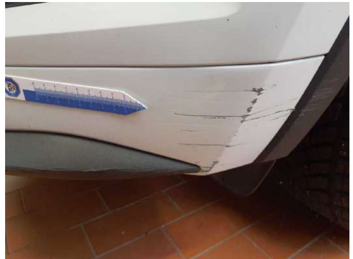
Damage 8: Front bumper: Spoiler - Scratched - Paint
