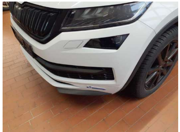
Damage 8: Front bumper: Spoiler - Scratched - Paint
