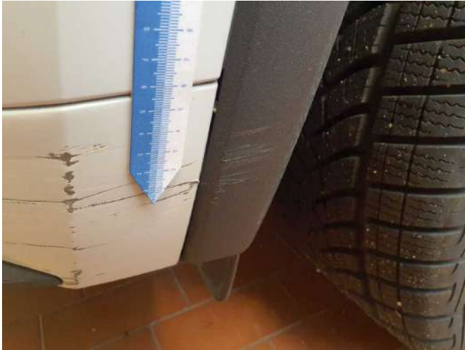
Damage 5: Mudguard - left side: Brightware, grille - Damaged - Replace
