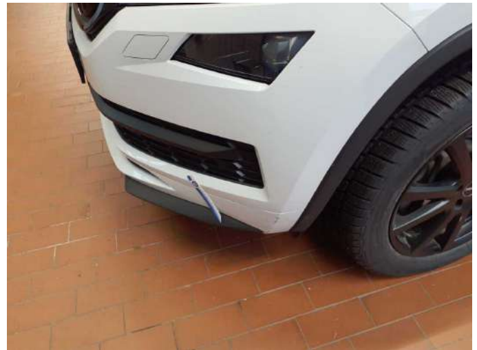
Damage 2: Front bumper: Cover bumper - front - Damaged - Replace
