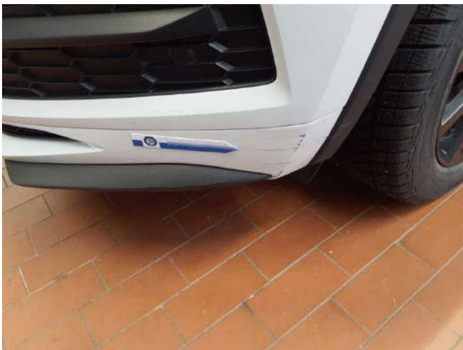
Damage 8: Front bumper: Spoiler - Scratched - Paint
