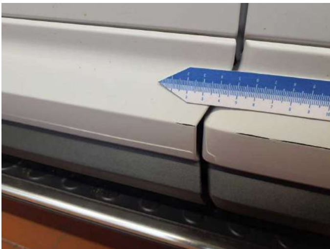
Damage 6: Door - front left side: Brightware - lower - Damaged - Paint
