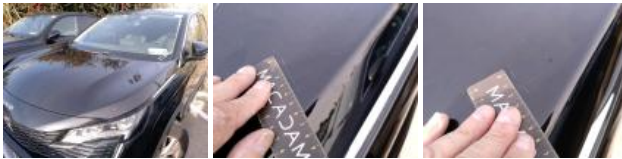
Bumper moulding F, Scratch(es), Replace
