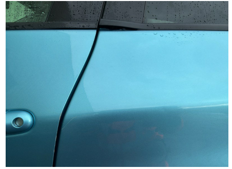
EXTERIOR - DRIVERS SIDE Door nsr; Scratched; UpTo 25mm Thru Paint
