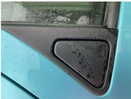
EXTERIOR - PASSENGER SIDE Handle Outer osr; Scratched (Painted); Up To 25mm Thru Paint
