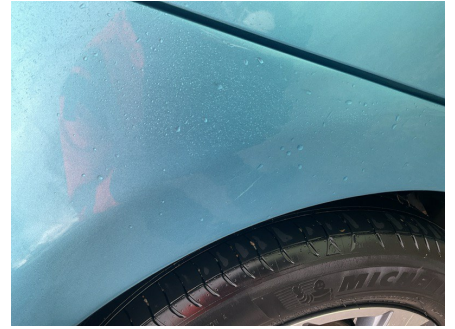
EXTERIOR - PASSENGER SIDE Qtr Panel osr; Scratched; Up To 25mm Thru Paint
