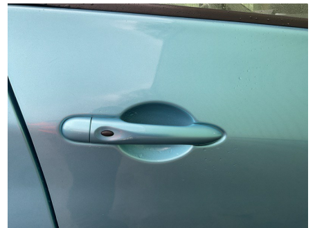
EXTERIOR - PASSENGER SIDE Door osf; Scratched; Up To 25mm Thru Paint
