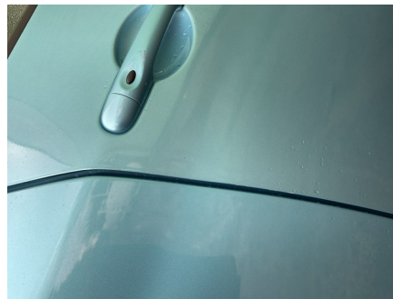
EXTERIOR - PASSENGER SIDE Door osf; Scratched; Up To 25mm Thru Paint
