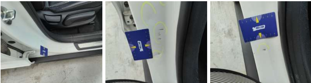
Rocker Panel Right // Smart Repair Medium-scratch + dent
