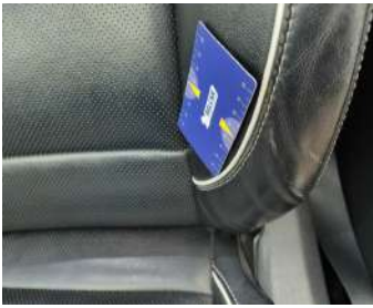
Seat Front Left / Complete Coating / Replace-worn
