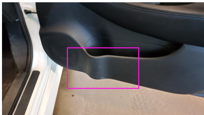
2. Door Step / Front Right Interior / Scratched
