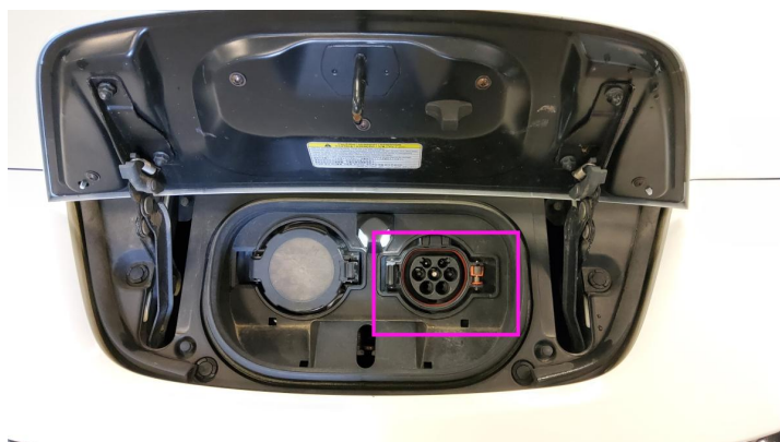
4. EV charging port
