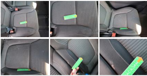
Seat cover FL, Tear, Repair/replace (lump sum)
