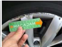
Tyre RL, Out of tolerance, Replace
