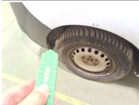
Wheel arch trim Front part / Front Left / Broken
