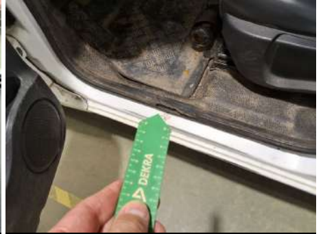
Door entry seal / Front Left / Tear
