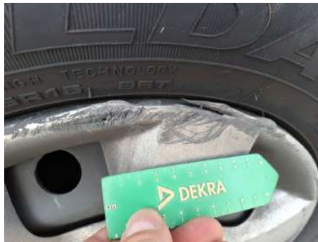
Wheel trim / Front Right / Broken
