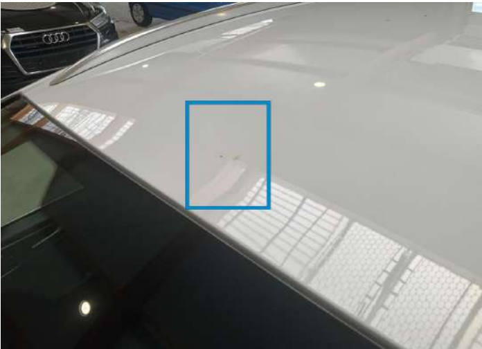
21. Roof Paint / Stone Chip -
