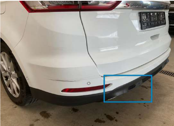
19. Bumper / Back Bodywork / Dent / Deformation -
