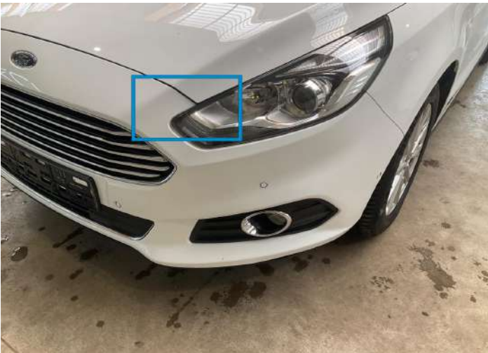
23. Bumper / Front Bodywork / Poor Previous Repair -
