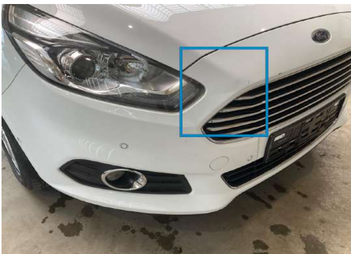
18. Bumper / Front Bodywork / Breakage / Hole -
