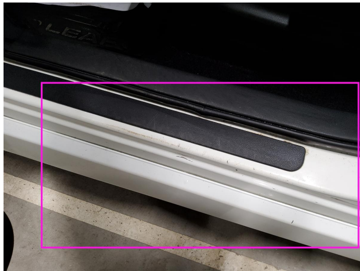
2. Door Step / Front Left Interior / Scratched
