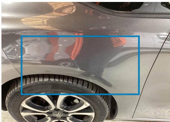
13. Fender / Front Left Bodywork / Dent / Dent -
