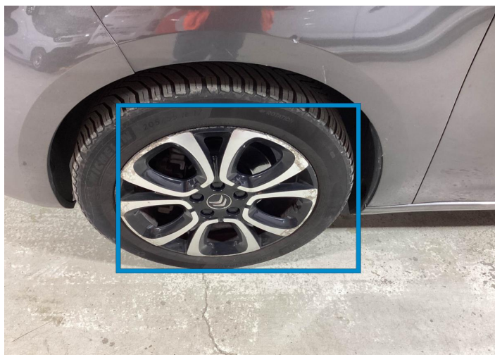
17. Rim / Front Left Out of Bodywork / Scratch -
