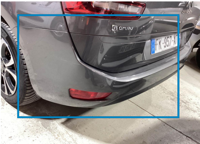
1. Corner Bumper / Back Left Paint / Scratch / Scuff -
