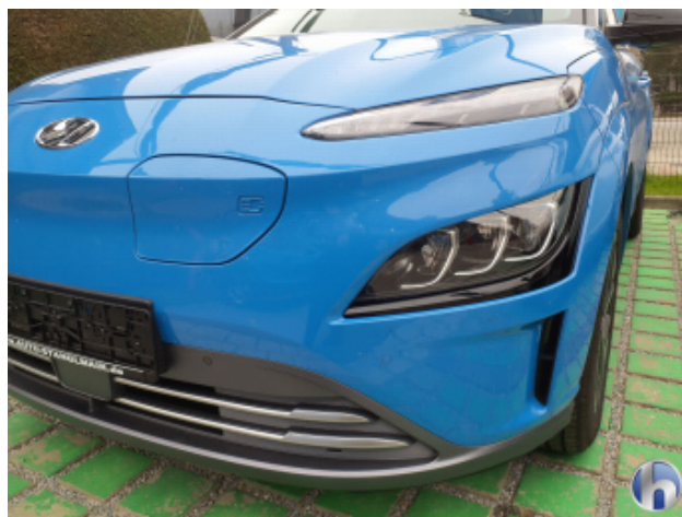
2. Front bumper Chipping from stones - Paint
