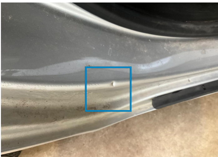
12. Door / Back Right Bodywork / Dent / Dent -
