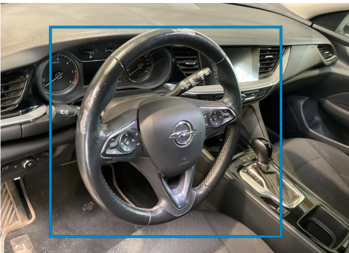
5. Steering Wheel / Front Interior / Worn - out -
