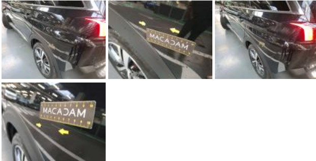
Central pillar moulding L, Scratch(es), Replace
