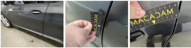
Roof pillar L, Dent(s), Repair and paint (complete)
