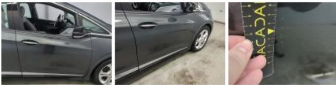
Door FR, Scratch(es), Repair and paint (complete)
