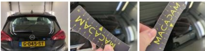
Rear spoiler, Scratch(es), Repair and paint (complete)
