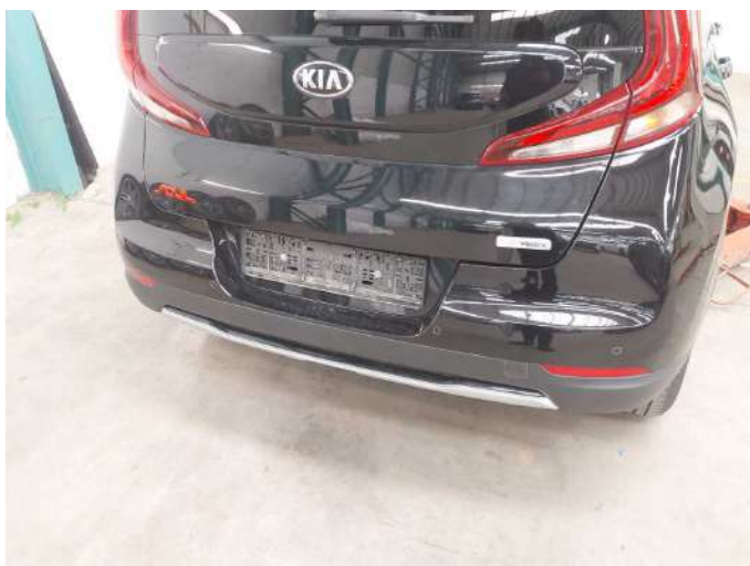
Damage 13: Rear bumper: Rear bumper - Scratch(es) - Paint
