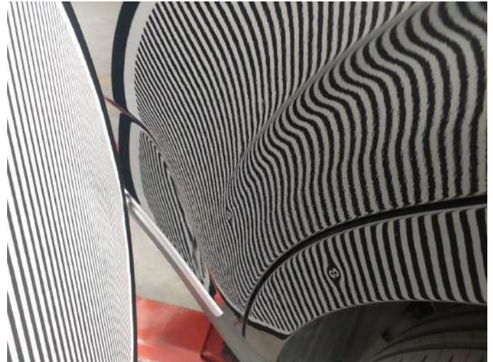
Damage 8: Door - rear left side: Door - dent(s) - Smart repair
