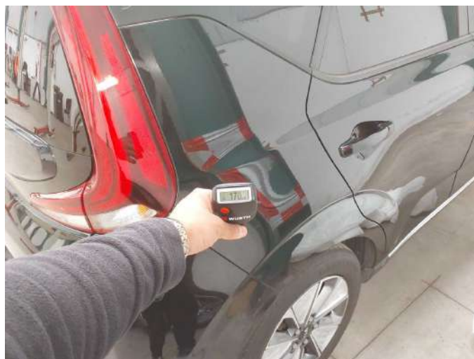
Side panel - rear right side: 170 \mu\text{m}
