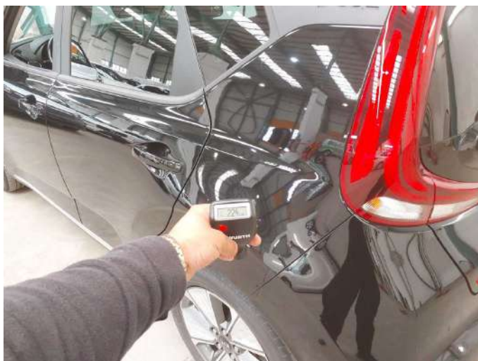
Side panel - rear left side: 224 \mu\text{m}
