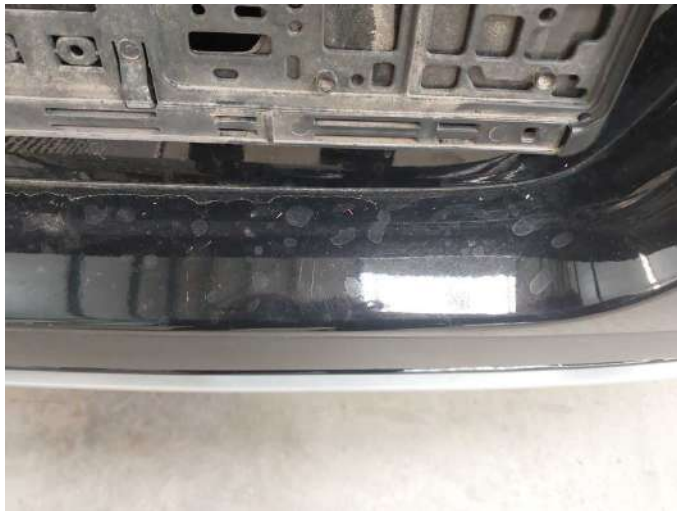
Damage 13: Rear bumper: Rear bumper - Scratch(es) - Paint
