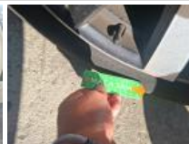
Tyre RR, Out of tolerance, Replace
