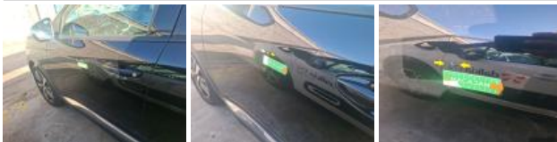
Side repeater L, Broken, Replace
