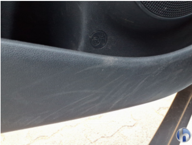
16. covering Wear and tear - Without repair
