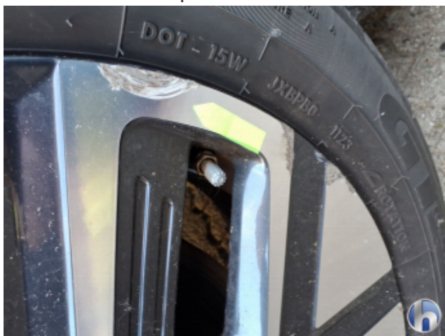
6. Rim front - left Damaged - Smart repair
