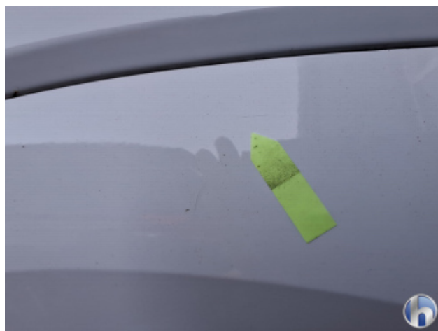
5. Sidewall - Rear - Left Deep scratch - Smart repair
