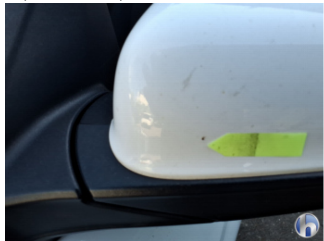
13. Outside mirror - left Chipping from stones - Smart repair
