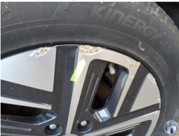
12. Rim rear - right Damaged - Smart repair
