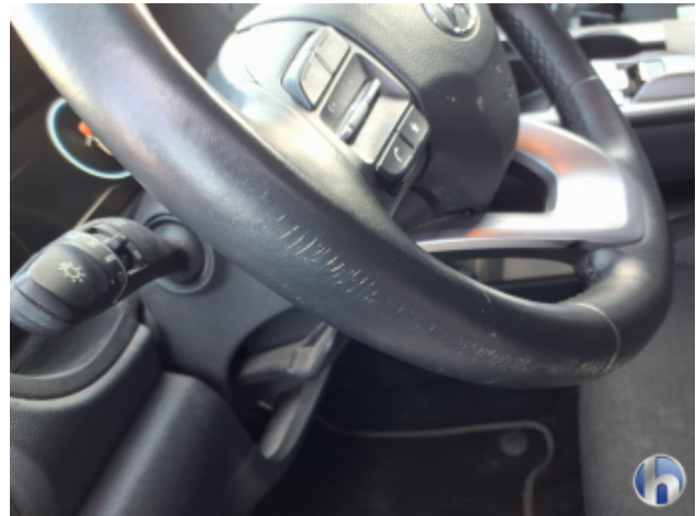
17. Steering wheel (leather) Deep scratch - Replace
