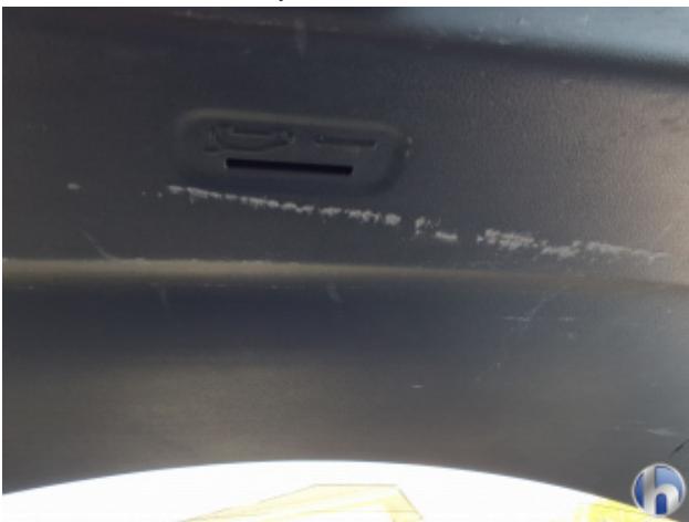
18. tailgate trim Damaged - Replace
