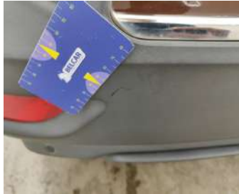
Bumper Rear / Lower Cover Not Painted / Replace-scratch
