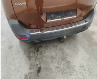
Bumper Rear / Lower Cover Not Painted / Replace-scratch
