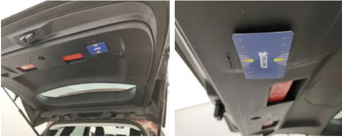
Trunk Lid Interior Coating / Complete Panel / Replace-scratch
