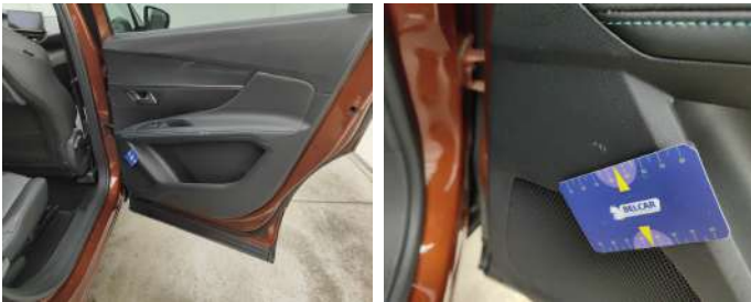
Rear Right Door Interior Coating // Replace Completely-scratch
