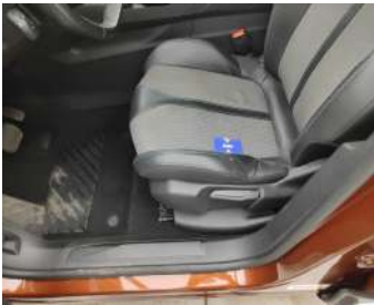
Seat Front Left / Bottom Coating / Replace-worn
