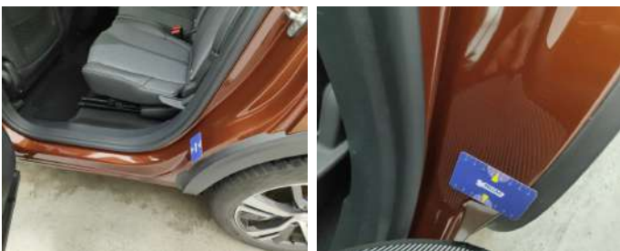
Rocker Panel Left // Smart Repair Medium-dent
