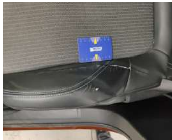
Seat Front Left / Bottom Coating / Replace-worn
