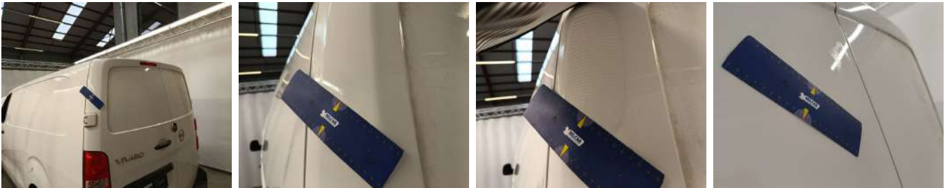
Rear Loading Door Left // Repair & Painting-bad repair
