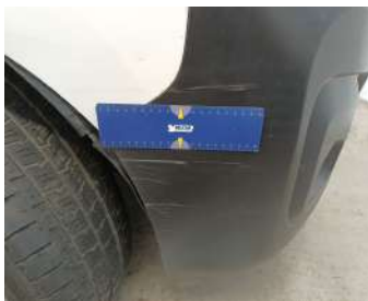
Bumper Front // Replace without painting-scratch
