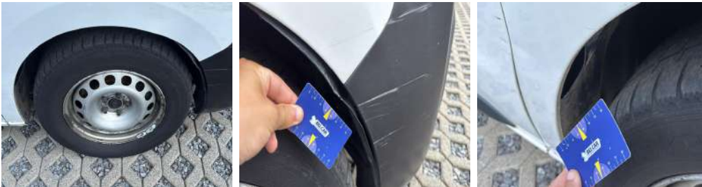
Wing Front right / Inner Fender / Replace-cracked
