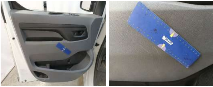
Front Left Door Interior Coating // Replace Completely-scratch
