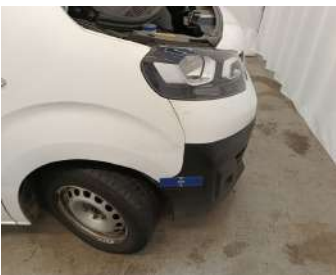
Bumper Front // Replace without painting-scratch
