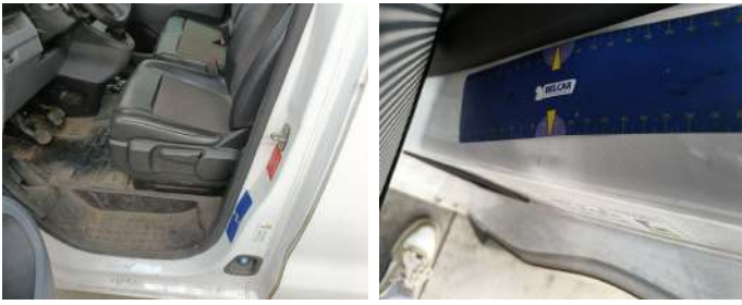
Rocker Panel Left // Smart Repair Medium-scratch + dent
