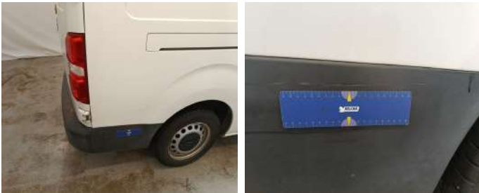
Bumper Rear // Replace without painting-scratch
