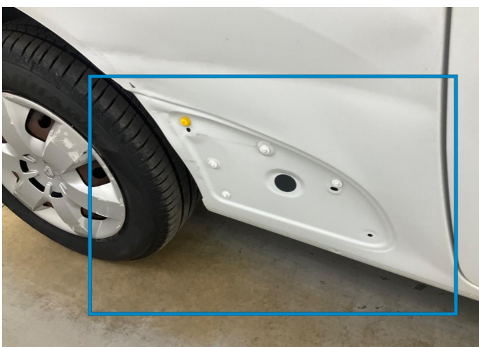
4. Fender / Back Right Missing Part -
