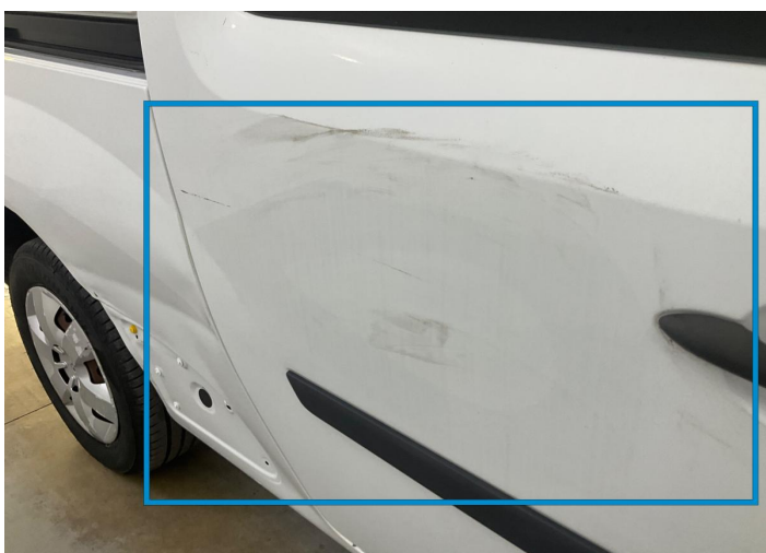
3. Pillar / Back Right Paint / Scratch / Line -
