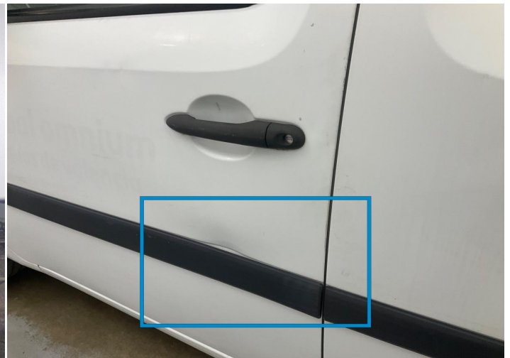
10. Door / Front Left Bodywork / Dent / Dent -
