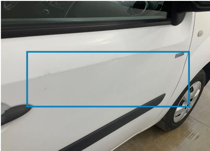
7. Door / Front Right Paint / Scratch / Line -
