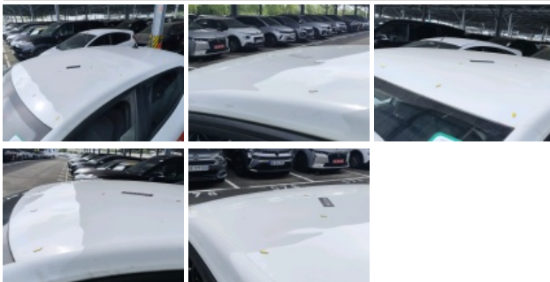
Roof, Dent(s), Repair and paint (complete)
