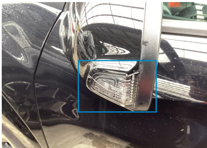
3. Mirror Repeater / Left Paint / Scratch / Line -
