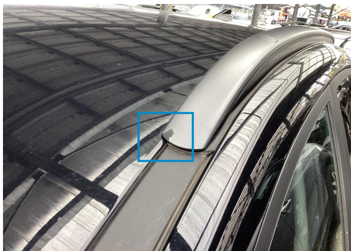
5. Roof Rack / Left Paint / Chipping -
