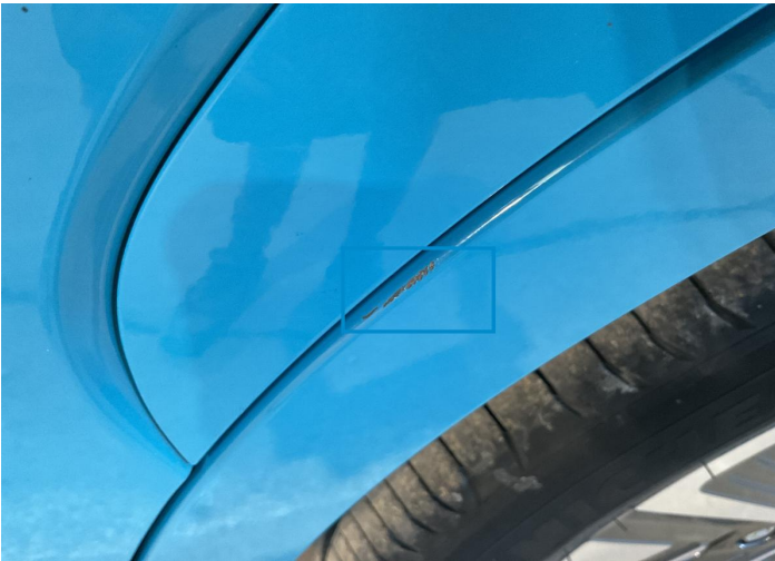
1. Mud Flap / Back Left Paint / Chipping -
