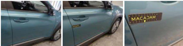
Door RR, Scratch(es), Repair and paint (complete)
