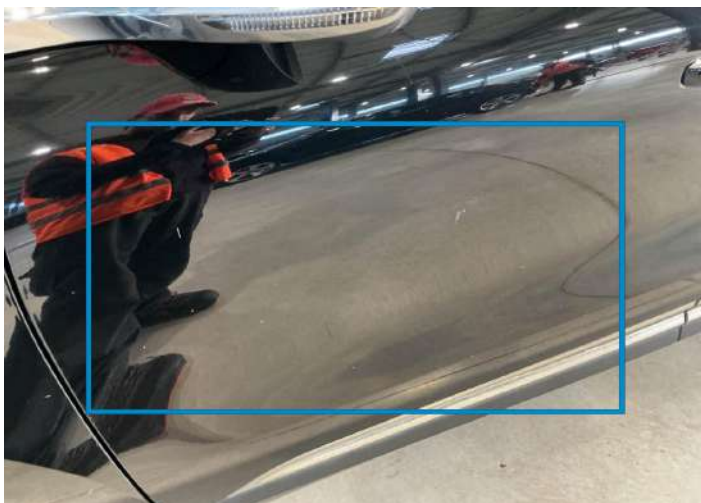
21. Door / Front Left Paint / Scratch / Line -
