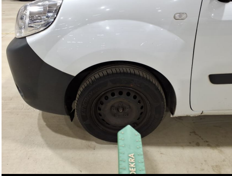
Wheel trim / Front Left / Missing
