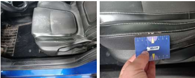
Seat Front Left / Bottom Coating / Replace-worn
