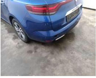
Bumper Rear // Replace & Painting-scratch + dent
