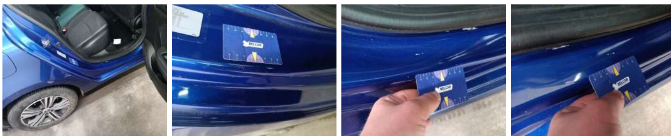
Rocker Panel Right // Smart Repair Medium-scratch
