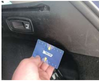
Trunk Lid Interior Coating / MDF Rear Right / Replace-scratch
