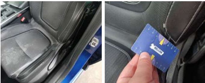
Seat Front Left / Rear Coating / Replace-worn
