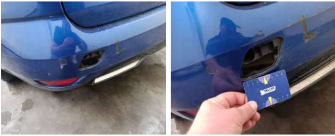
Towing Cover Rear // Replace-missing
