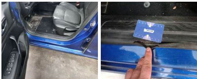
Door Front Left / Trim / Replace-cracked
