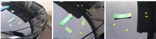
Door FR, Bad repair, Paint
