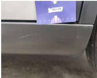
Rocker Panel Left / Cover Not Painted / Replace-scratch
