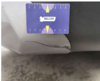
Bumper Front / Spoiler / Replace-scratch
