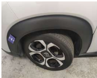
Wing Front Left / Trim / Replace-scratch
