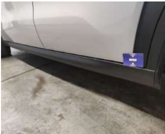
Rocker Panel Left / Cover Not Painted / Replace-scratch
