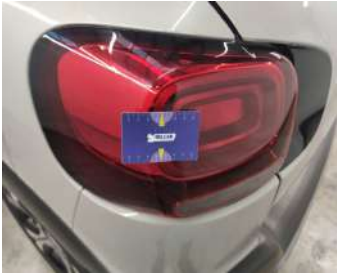
Light / Rear left / Replace-scratch
