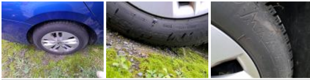
Tyre FR, Out of tolerance, Replace
