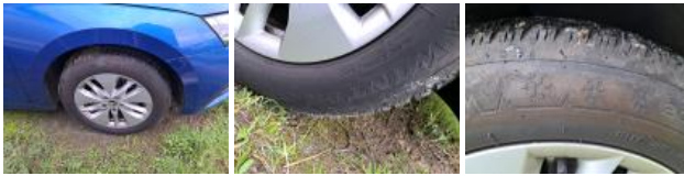
Tyre FR, Out of tolerance, Replace
