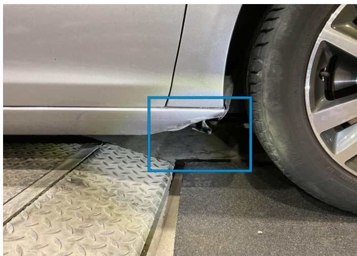
5. Rocker Panel / Center Right Bodywork / Dent / Deformation -
